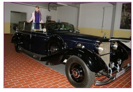
Presumed Hitler 770 is from the 1st series constructed from 1930-1938 and carried 7.65 liter straight eight fitted with a Roots type supercharger. With 18 mm armor protection and bullet-proof glass, this 770 was a heavyweight.
